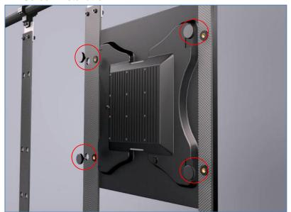
1.Fix XMOZU panel on carbon fiber board with black POM gasket (integrated with screws.)
