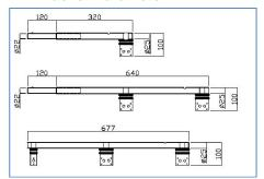
1. Carbon Fiber Tube length:677mm,640mm,320mm
