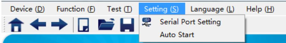
**[Serial Port Setting]:**Configure the serial ports connecting the control system and computer
